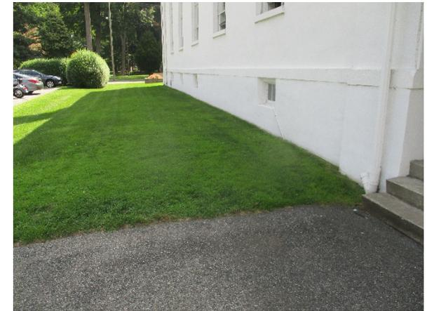
Bioretention systems can be installed north and south of the church building to capture, treat, and infiltrate stormwater runoff from the rooftop. A preliminary soil assessment suggests that more soil testing would be required before determining the soil's suitability for green infrastructure.
