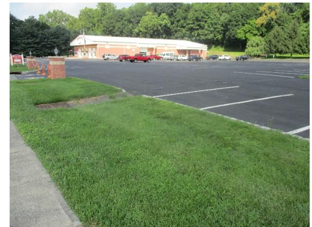
Pervious pavement can be installed west of the building on the southernmost parking strip to capture, treat, and infiltrate stormwater runoff from the parking lot. Bioretention systems can be installed in the turfgrass area between the parking lot and sidewalks to intercept stormwater before it enters the catch basin storm drains. A preliminary soil assessment suggests that more soil testing would be required before determining the soil's suitability for green infrastructure.
