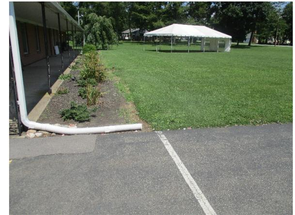
Two bioretention systems can be installed to the north and west of the building to capture, treat, and infiltrate stormwater runoff from the roof using the disconnected downspouts. A preliminary soil assessment suggests that the soils have suitable drainage characteristics for green infrastructure.
