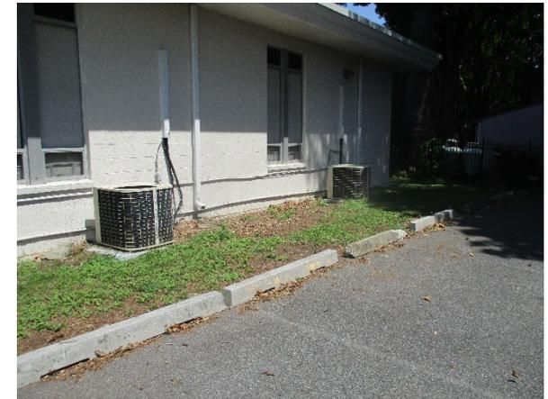
Two bioretention systems can be installed north of the building to capture, treat, and infiltrate stormwater runoff from the roof. Downspout planter boxes can be installed on the south end of the building to capture rooftop runoff to reduce stormwater flow onto the pavement. A preliminary soil assessment suggests that the soils have suitable drainage characteristics for green infrastructure.
